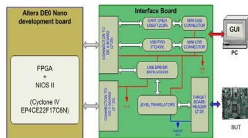
Figure 1. Hardware Architecture
