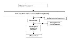
Fig. 1.3 Practical Ballooning and Routing Process
