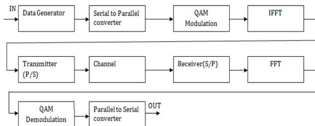
Fig 1. The Basic Model of OFDM System
