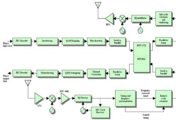
Fig 2. Block Diagram of an OFDM Transceiver:
