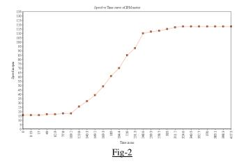
The figures (2) and (3) shows the speed and torque characteristics of a 2kW IPM motor at various frequencies.
