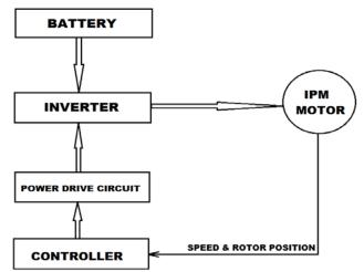
Fig.1 Block diagram showing Electric Propulsion System in Electric Vehicle
