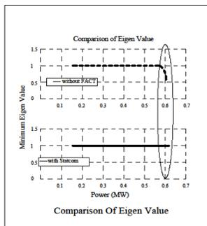
The Point of Placement of Controller (STATCOM)
