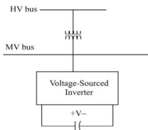
STATCOM is used to provide reactive power to the ac system, beside that, it will provide the dc power required for
