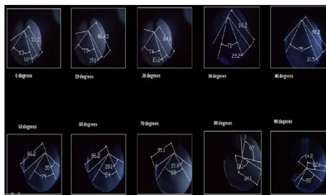
Fig.4.2 Spray Cone Angle, Dispersion Angle and Penetration Lengths Of 950ml Diesel and 50ml Ethanol at various Injector Angles
