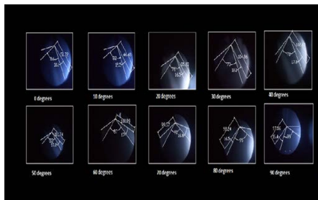
Fig.4.1 Spray Cone Angle, Dispersion Angle and Penetration Lengths Of 1000ml Diesel at various Injector Angles
