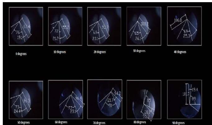
Fig.4.4 Spray Cone Angle, Dispersion Angle and Penetration Lengths Of 850ml Diesel and 150ml Ethanol at various Injector Angles
