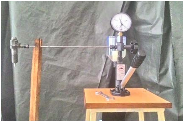
Fig.2.2 Fuel Injector Testing Equipment
