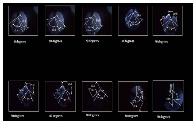
Fig.4.3 Spray Cone Angle, Dispersion Angle and Penetration Lengths Of 900ml Diesel and 100ml Ethanol at various Injector Angles
