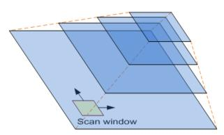
Fig. 2. 2 Scan-window and image pyramid
