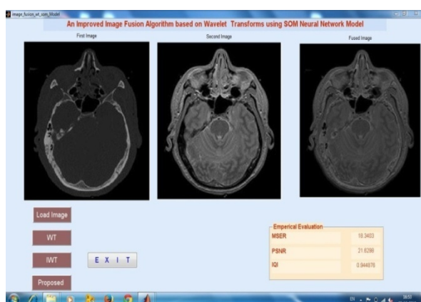
Figure 12: Shows that the fused Image obtained after fusion of BHCT1 & BHMRI1 images for the method Integer Wavelet Transformation(IWT) and values of MSER, PSNR and IQI.
