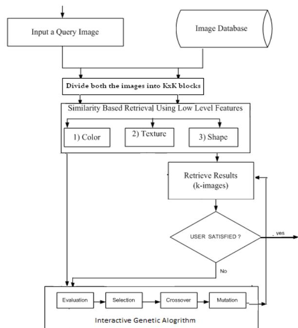
Figure (1): Improved Content Based Image Retrieval System Using IGA Approach
