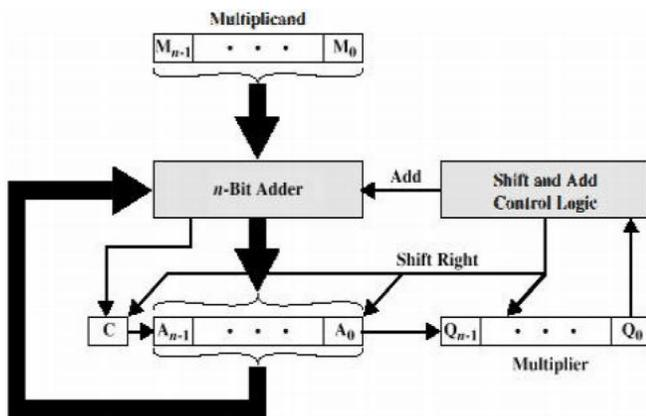
Fig. 2.1 Multiplier of two n-bit values
