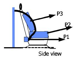
From figure, P1 &P3 are load at upper & lower belt anchorage point. P2 is 20 times weight of overall seat structure.so that P1, P2 & P3 have some load value that is 13518N for P1 & P2 both.
