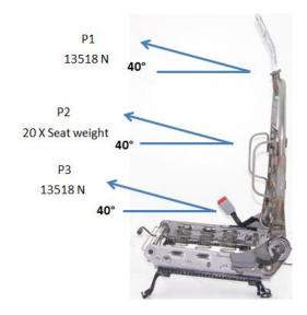
**1.1.Requirement:-**Belt anchorages must withstand specified load at least 0.2 second & no part to deform in such a manner as to present any hazard to occupant. During test no track tilt and latching must not disengage during the test
