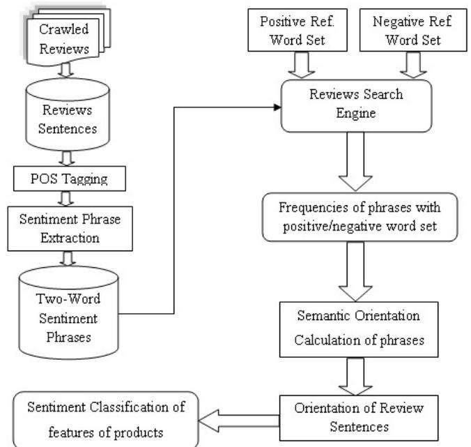
Fig. 1.1 Architectural Overview of Semantic Orientation System
