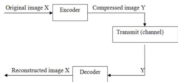
Fig. 1 Block diagram of image compression model
