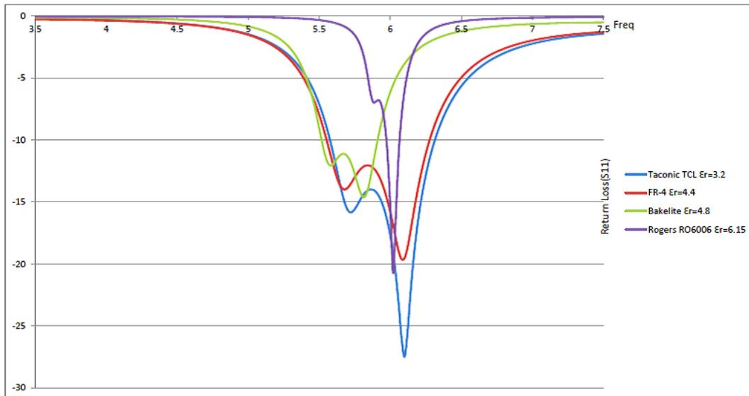
Figure 3: Return loss curves for different substrate materials.
