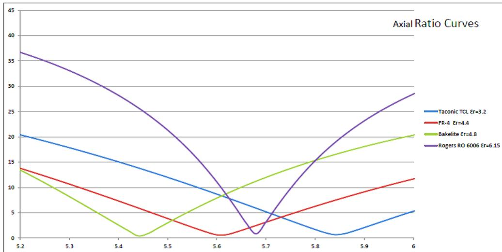
Figure 2: Axial ratio curves for different substrate materials.
