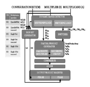
Figure 2.2 Block diagram of the Configurable Booth Multiplier
