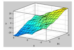
Fig.4.1 Surface view of input and output of the fuzzy inference
