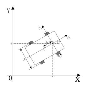
Fig.2.1 Motion diagram structure model of the power substation inspection robot
