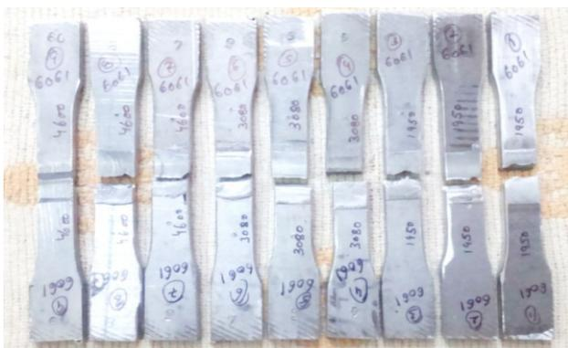
Fig. 3.8 Tensile test specimen after failure
