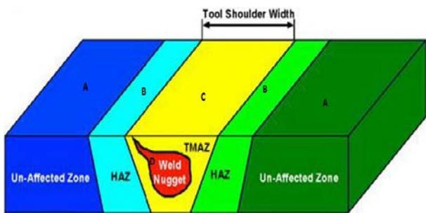
Fig. 3.2 Different types of Zone's made during welding
