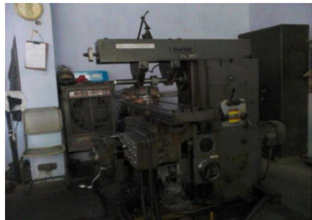
Fig. 3.6 Horizontal milling machine
