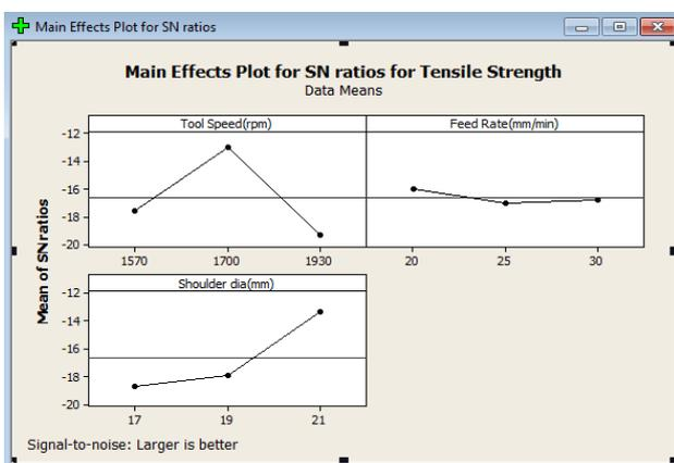
Fig. 3.9 Main effects plot for SN ratio for Tensile Strength
