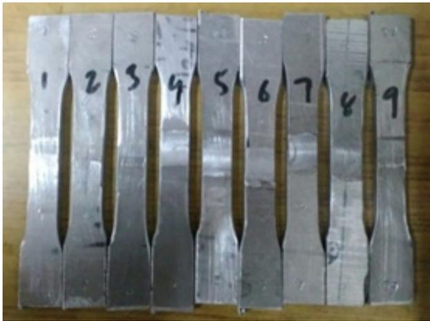
Fig. 3.7 Tensile test specimen before failure
