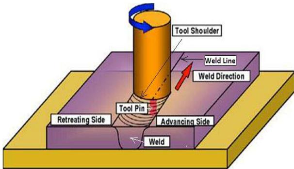
Fig. 3.1 FSW Process
