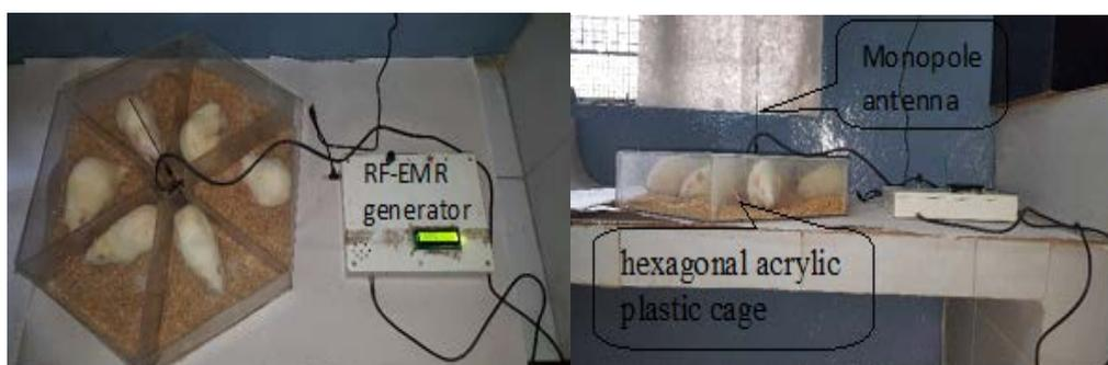
**Fig.1:** Male Wistar rats under RF-EMR exposure placed in hexagonal acrylic cage by placing the monopole antenna in the center of the cage.
