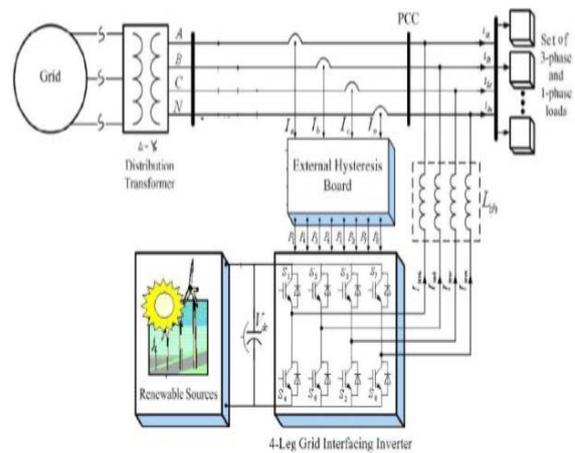
**Fig.1: 4 Leg grid interface unit**
