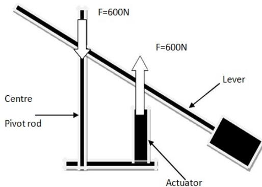
The approximate force applied by the human muscular force is taken into consideration and the force required in order to uproot the crops from the soil is determined. Hence the force assumed and the further calculations is as follows:-
