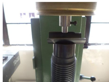
Fig 12: specimen mounted on hardness tester
