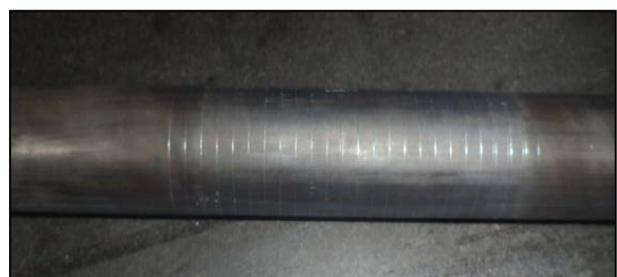
Fig 13: Induction hardened fork tube as specimen used for check of hardness after induction hardening.
