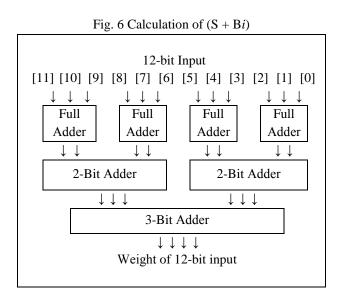
Fig. 7 Architecture of Weight Calculation Unit. Simplified adder based architecture is implemented in this work to calculate the weight of a 12-bit (S + Bi) and (SB + Bi), for  $1 \le i \le 12$ . The architecture of adder based weight calculation unit is shown in fig. 7.
