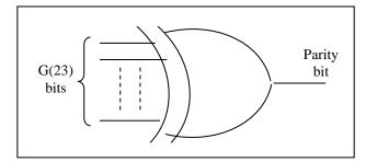
Fig 4 Parity Bit Generation using XOR-ing operation
