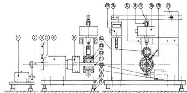
Fig.1 (Schematic diagram of the test rig for applying static and dynamic loads to journal bearing)
