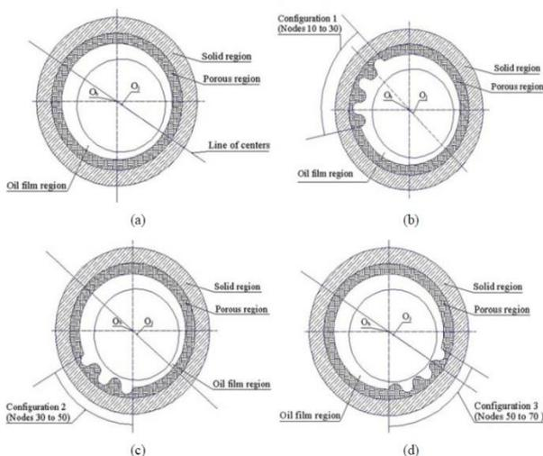
Fig.2 (Schematic representation of smooth porous journal bearing, (b), (c) and (d) surface texture at configurations 1, 2 and 3, respectively)
