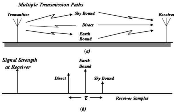
Figure 1.2 Impulse Response of a transmitted signal in a channel which has 3 modes of propagation, (a) The signal transmitted paths, (b) The received samples
