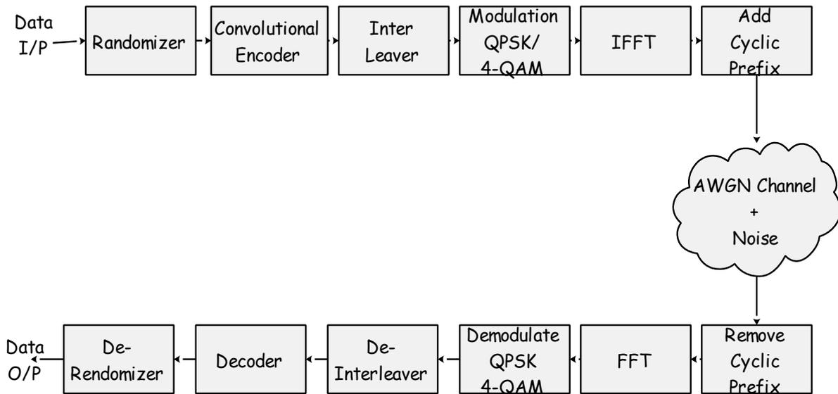
Figure 3.1 Block diagram of the Proposed System.
