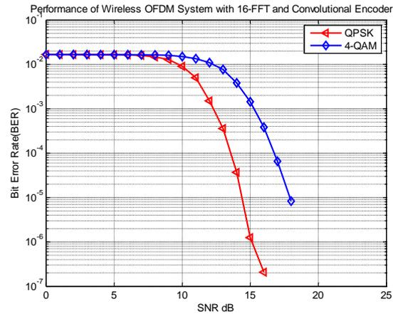
Fig. Proposed System Performance using 16-FFT using Convolutional Encoder with PSK and QAM Modulation
