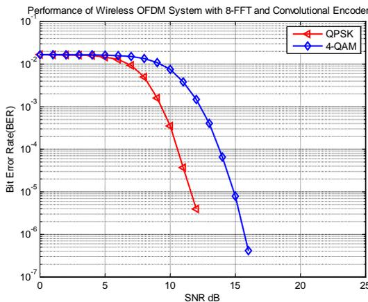
Fig 4.2 . Proposed System Performance using 8-FFT using Convolutional Encoder with PSK and QAM Modulation
