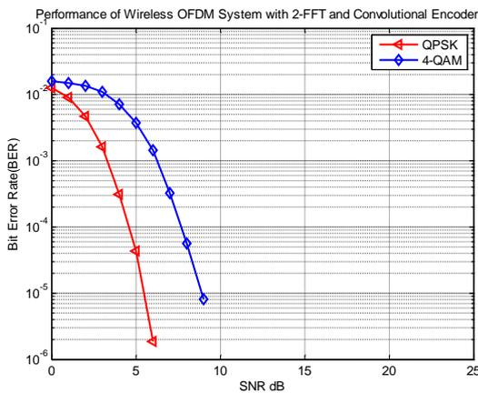
Fig 4.1 Proposed System Performance using 2-FFT using Convolutional Encoder with PSK and QAM Modulation
