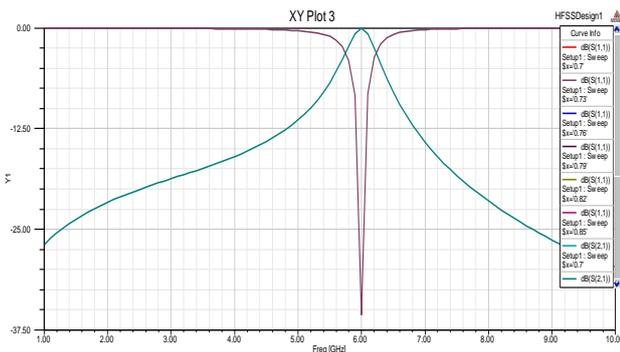
Fig. 4.2 Common graph for transmission band and return loss for single pole hair pin filter.
