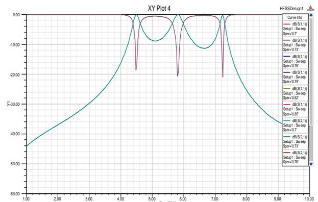
Fig. 4.4 common graph for transmission band and return loss for three pole hairpin filter
