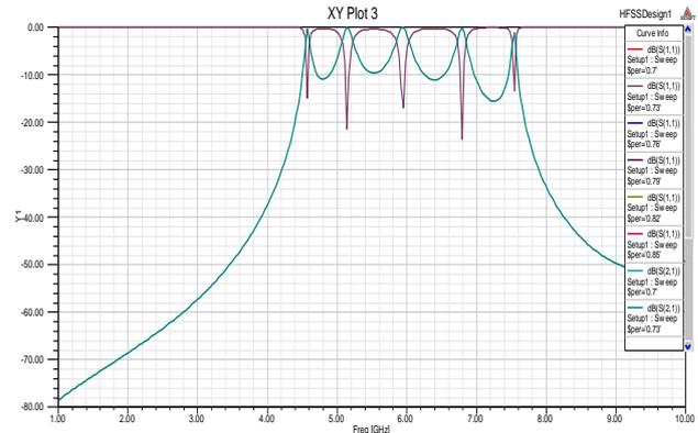
Fig. 4.6 common graph for transmission band and return loss for five pole hairpin bandpass filter.
