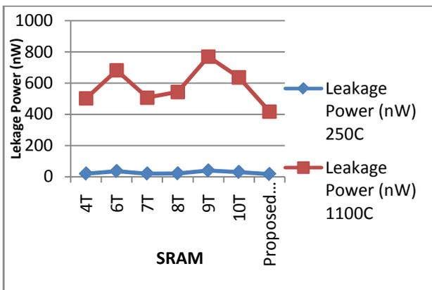
Fig. 6.3 Leakage power consumption of existing and proposed SRAM cell at 25°C & 110°C.
