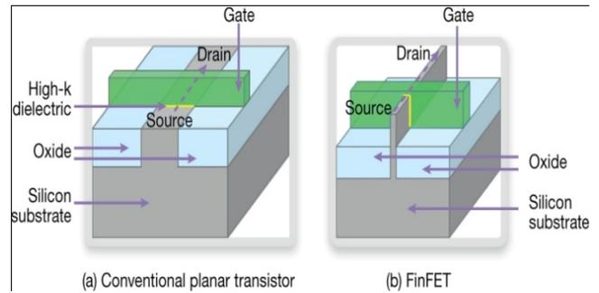
Fig. 4 (a) Conventional Planer Transistor (b) FinFET transistor, adapted from.
