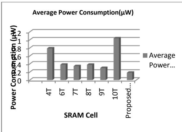
Fig. 6.2 Average power consumption of existing and proposed SRAM cell.
