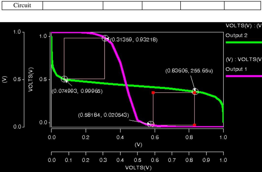
Fig. 6.1 SNM Butterworth Curve of Proposed 9T SRAM Cell.
