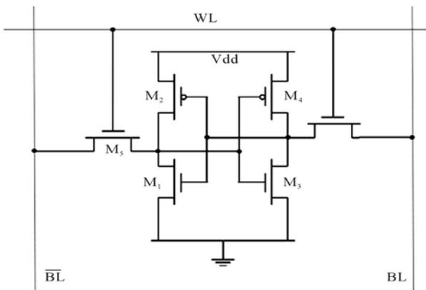
Fig. 3. Conventional 6T SRAM cell
