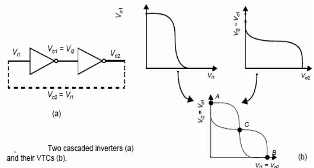
Fig. 1 Back to back connected in- (c).
