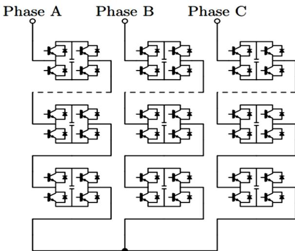
Figure 2.1 The circuit of Cascaded Multilevel Converter.
