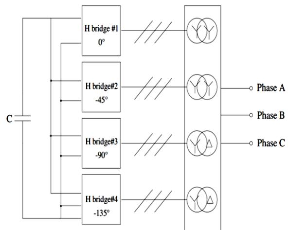
Figure 2.2 The circuit of transformer phase-shifted cascaded H bridge converters.
