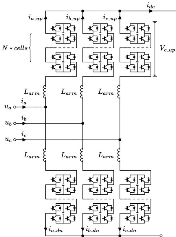
Figure 2.3 MMC topology with a full-bridge cell configuration
