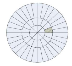
Fig. 1.3 The tiling of polar frequency domain. The shadowed 'wedge' corresponds to the frequency transform of the element function.
