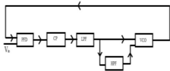
Figure.1 block diagram of the Novel Flash Locking DPPLL
