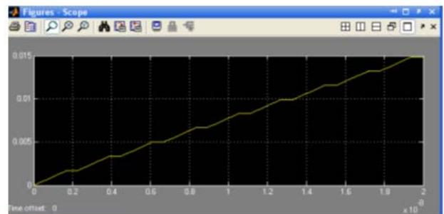
Figure 6-Third order Charge pump PLL filter output
