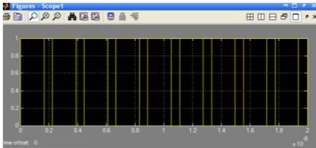
Figure7-Third order Charge pump PLL Phase detector output
