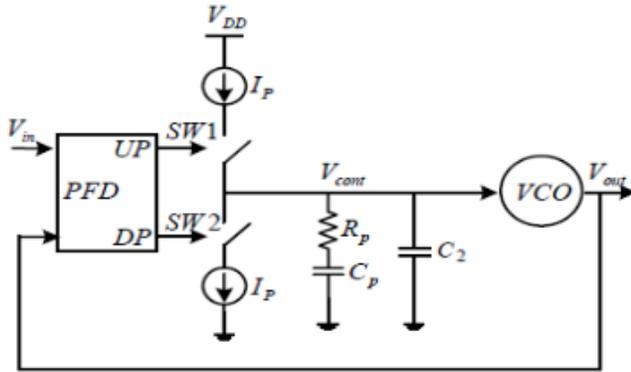
Figure 4- Structure of third order charge pump DPLL
