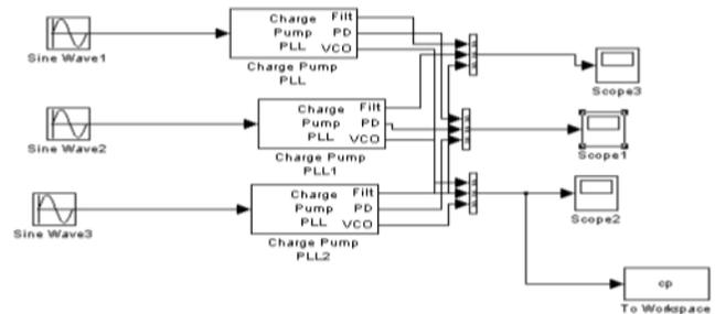
Figure9- Setup for measurement of PLL parameters in Simulink
