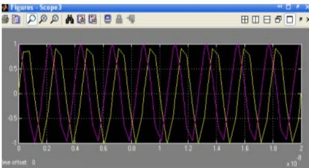
Figure-8 Third order Charge pumps DPLL VCO output and input signal
