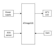
The detector made use of a user friendly, portable and easy to handle are design and development perspective. In the system consists of a micro controller board, ECG sensor, transformer, bridge rectifier, input capacitor 7805 for regulated power supply 16\*2 LCD.
