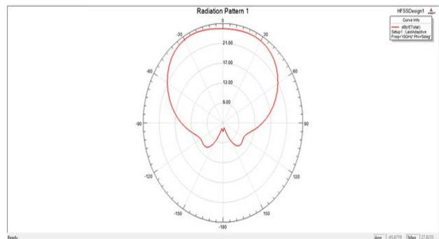
Figure 6: Radiation pattern of the microstrip patch antenna
