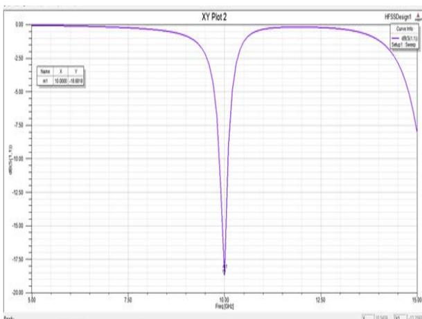
Figure 4: Plot between S (11) Vs Frequency
