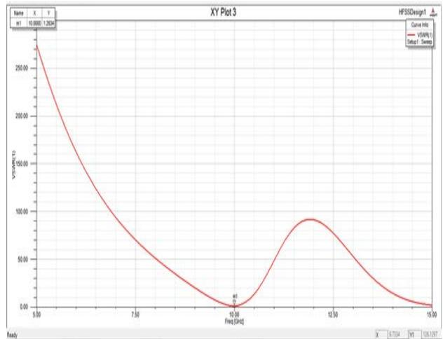
Figure 5: Plot between VSWR Vs Frequency
