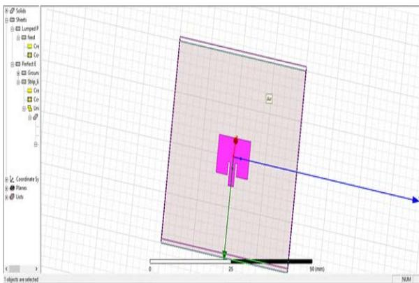
Figure 3: Diagram of the microstrip patch antenna
