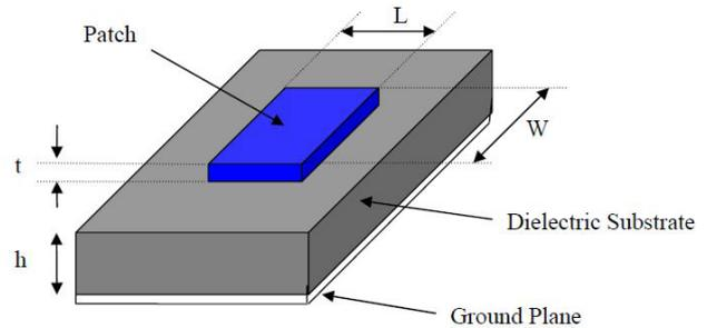
Figure 2: Microstrip patch antenna
