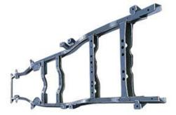
Fig 1:Ladder frame chassis
