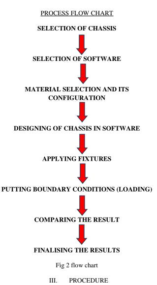
The whole procedure included the formation of the **TOYOTA INNOVA 2.5G (2014)** chassis in solidworks software. Afterwards that several types of analysis are done on it. The results from this chassis are considered and after that making
