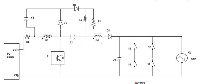
Fig.3 Circuit diagram of modified luo converter with coupled inductor
