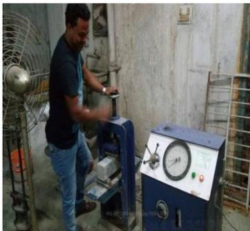
**Figure-6: Experimental Setup for Flexural Strength**
