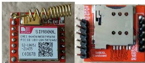
Fig. 5.1 GSM modem
