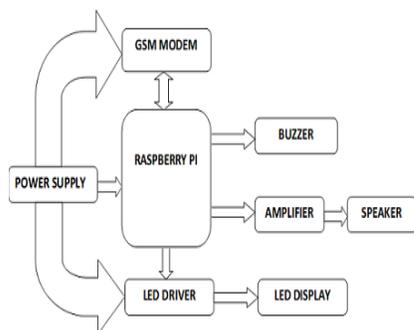
Fig 3.2 Block diagram of Digital notice board using Raspberry pi
