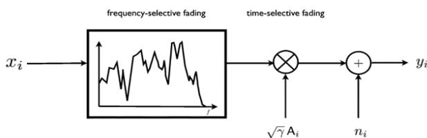
Fig. 2.1 block diagram of frequency selective channels.
