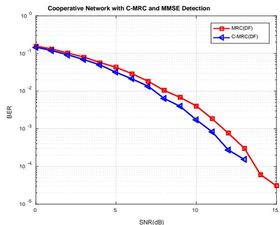
Fig. 4.2 BER Vs SNR Curves using Relay Selection and MMSE Detection Relay Selection with MMSE Detection, Different Combining Techniques and Cooperative Modes
