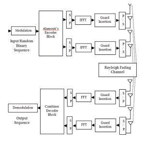
Figure 1: System Model of MIMO-OFDM system
