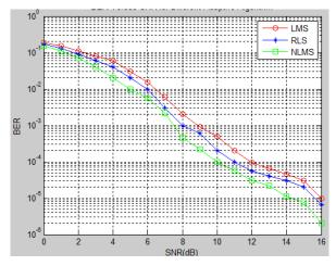
Figure 7: Performance BER versus SNR in Different Adaptive Algorithm
