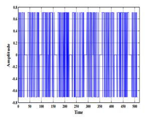
Figure 2: Transmitted QPSK symbol of MIMO-OFDM  $(N_{Tx} \times N_{Rx}) \text{ system}.$
