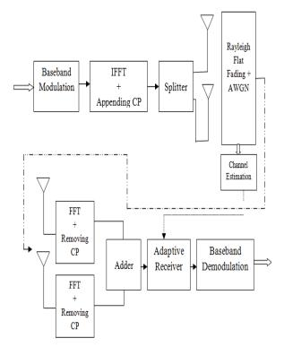
Figure 4: 2x 2 MIMO-OFDM System Models with Adaptive Filter
