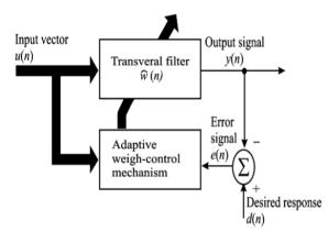
Figure 3: Block diagram of adaptive transversal filter
