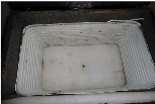
Fig.3.1 Evaporating Coils
