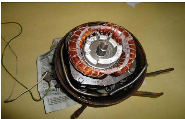
Fig.3.2 Compressor Coils Winding
