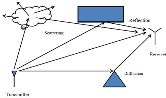
Fig. 2.1: Different Paths in Wireless Channel
