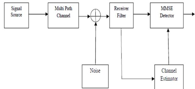
Figure 3.1: Block Diagram of a Noise-Corrupted System with MMSE Estimation
