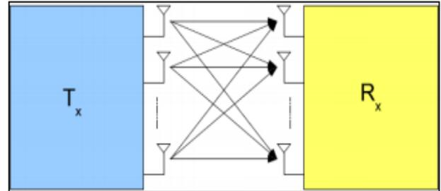
Fig. 1.1: MIMO Communication System
