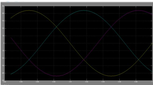
Fig.6 Output voltage of three-phase transformer with continuous.
