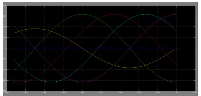
Fig.10 Output current of five-phase transformer with continuous.
