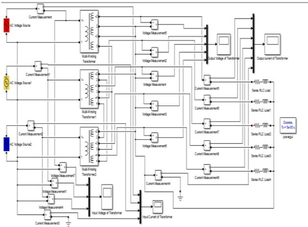
Fig.4 MATLAB simulation model of the three-phase to five-phase transformer.
