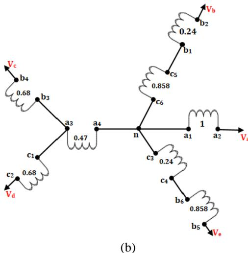
Fig.2. (b) Proposed transformer winding connection (star).
