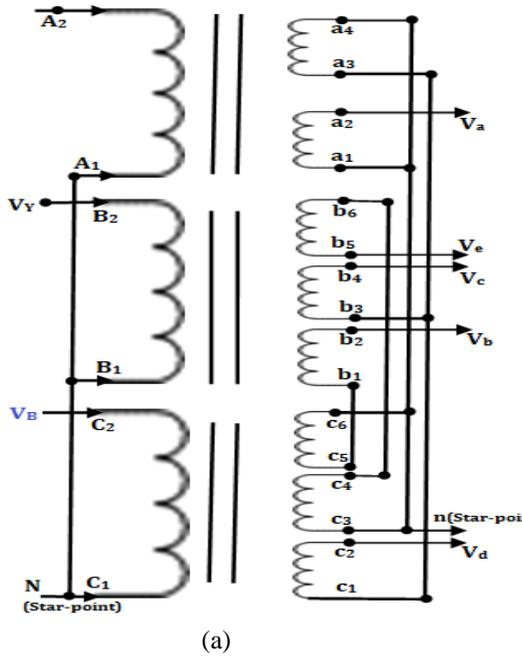
Fig.2. (a) Proposed transformer winding arrangements (star-star).
