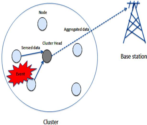
Fig. 2.1 a Basic Clustering Sensor Network.
