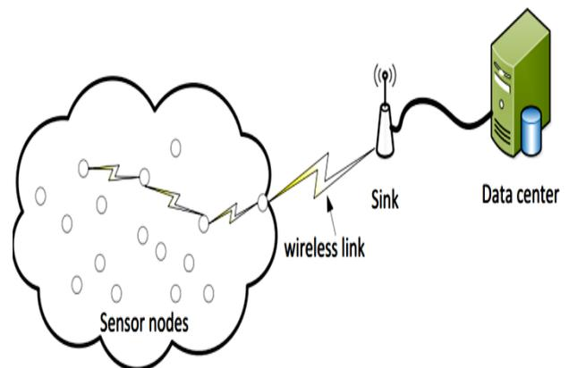
Fig. 1.2 General architecture of wireless sensor network
