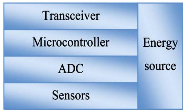
Fig. 1.1 Architecture of a sensor node
