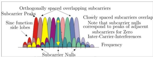
Fig. 1.1 OFDM Signal Frequency Spectra.
