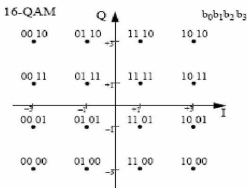
Fig. 3.2 Constellation Diagrams for 16 QAM.
