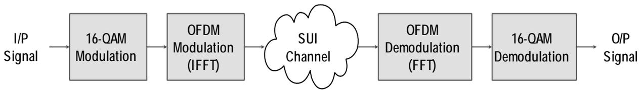
Figure 3.1 Block Diagram of Proposed System.
