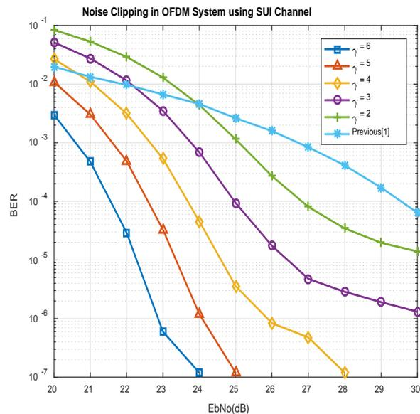
Fig.4.1 Bit Error Rate Performance of the proposed Methodology.
