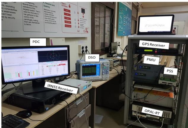
Figure-4: RT-HIL testing of hardware prototype of damping controller
