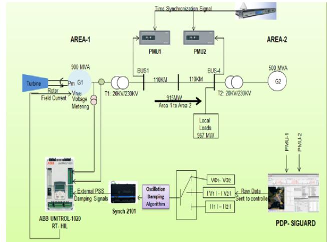
Figure-1: 2-area 2-machine model. G1 is equipped with Unitrol 1020 AVR .
