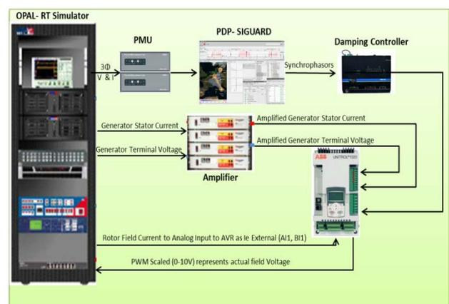
Figure-2: Interfacing Unitrol 1020 AVR with RTS and WADC.
