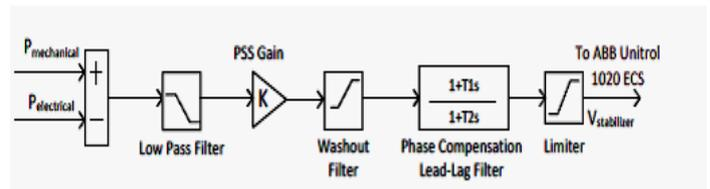
Figure-9: Model of conventional  $\Delta Pa$  PSS.
