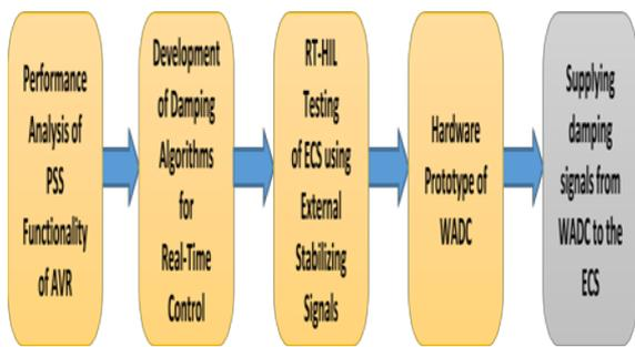
Figure-3: Steps involved in the development of Damping Controller based on wide area monitoring
