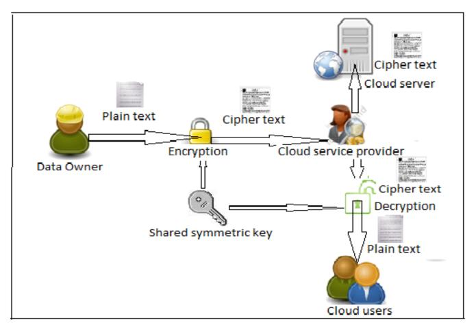
Fig: Block Diagram of Data Encryption and decryption in cloud system.
