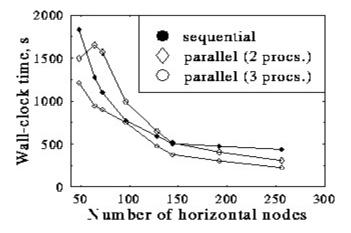
Fig.3 Execution time of parallel program on networked RS63 vs. number of processes; mesh: 256 x 9 nodes; algorithm I.
