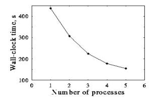
Fig.2 Execution time of sequential and parallel program on networked RS63; meshes with 2304 nodes; algorithm I.
