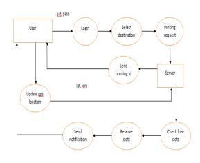
Figure 4: Level 2 Dataflow Diagram.
