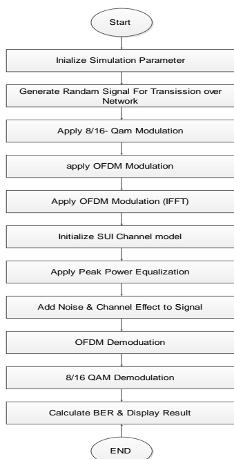
Figure 3.2 flow chart of 8 and 16 QAM modulation and demodulation
