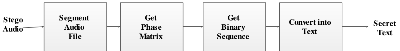
Fig.3.3 Block Diagram of Extraction Process.
