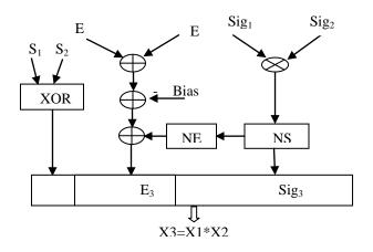
Figure 2: IEEE754 SP FP and DP FP Multiplier Structure, NE: Normalized exponent, NS: Normalized Significant
