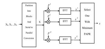
Figure 3: Block diagram of conventional SLM-OFDM transmitter
