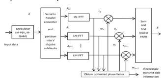
Figure 2: Block diagram of the PTS scheme with two transmit antennas
